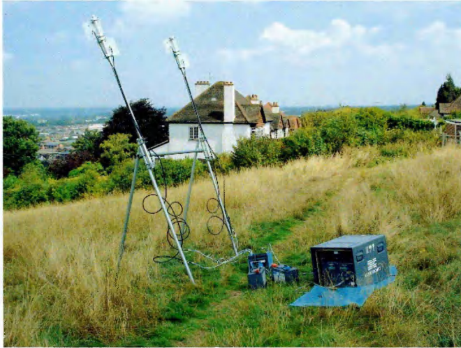
Fig. 5-4 Hill-mounted artificial platform showing antenna mast and sounder
